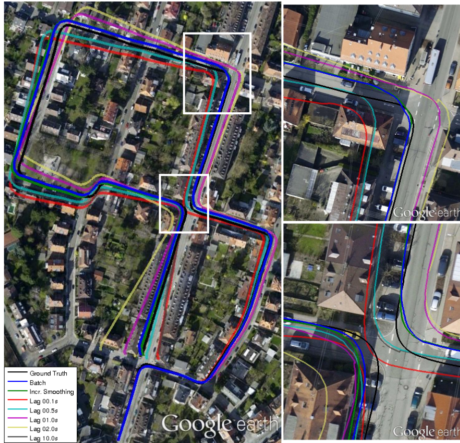
Figure 10: Trajectories for the ground truth, full batch optimization, incremental smoothing, and fixed-lag smoothers with lag sizes of 0.1, 0.5, 1.0, 2.0 and 10.0 seconds.
