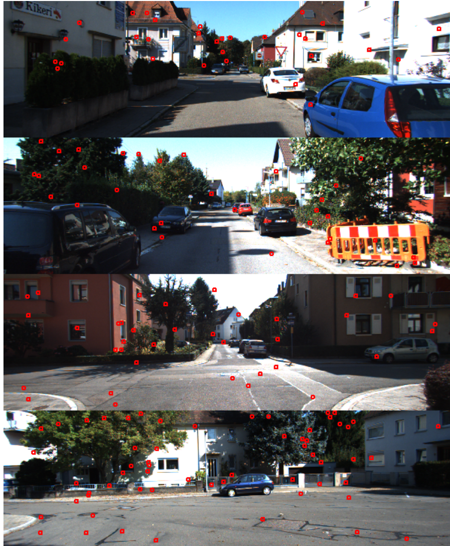
Figure 9: Typical camera images from the test KITTI dataset. Features tracked by the visual odometry system are indicated in red.
