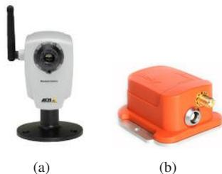
Fig. 14. Hardware used in the experiment. (a) Axis 207MW camera. (b) Xsens MTi-G IMU/INS.
