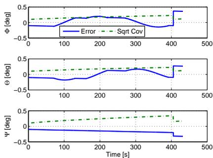
Fig. 12. Three-view method: a single loop update based on real images - Euler angle errors
