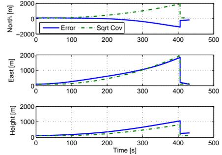
Fig. 10. Three-view method: a single loop update based on real images - Position errors
