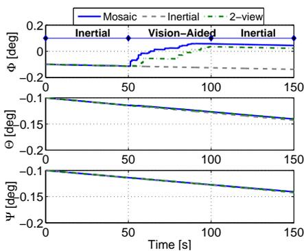
Fig. 5. Mosaic aiding applying two-view techniques vs. conventional two-view aiding: Euler angle errors. Roll angle error estimation for both motion estimation methods. Pitch and yaw angles errors are not reduced due to lack of observability.
