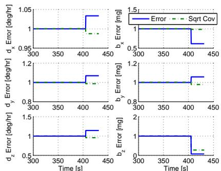
Fig. 13. Three-view method: a single loop update based on real images - Drift and bias estimation errors (zoomed)
