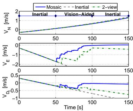
Fig. 4. Mosaic aiding applying two-view techniques vs. conventional two-view aiding: Velocity errors. Inertial error development in the north direction due to lack of observability. Reduced errors in the east and down directions, with a significant improvement in favor of the mosaic aiding.
