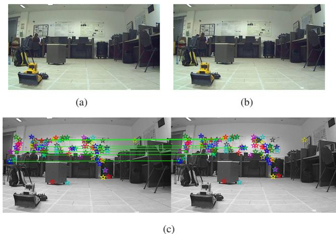
Fig. 17. Image matching process. (a),(b) Two camera-captured overlapping images. (c) Matching pairs:  $(\mathbf{x}_1, \mathbf{x}_2) \in \{\mathbf{x}_1^i, \mathbf{x}_2^i, \mathbf{x}_3^i\}_{i=1}^{N_{123}}$ . For clarity, only the first few matches are explicitly shown; the rest of the matches are denoted by marks in each image.
