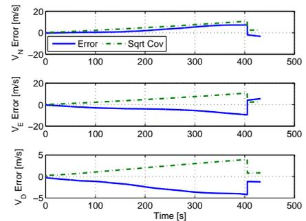
Fig. 11. Three-view method: a single loop update based on real images - Velocity errors
