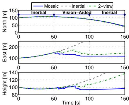
Fig. 3. Mosaic aiding applying two-view techniques vs. conventional two-view aiding: Position errors. Inertial error development in the north direction due to lack of observability. Reduced errors in the east and down directions, with a significant improvement in favor of the mosaic aiding.
