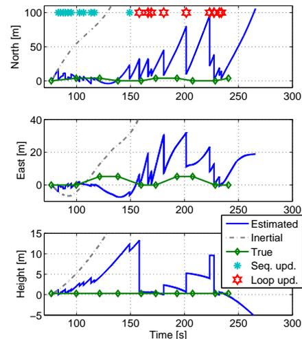
Fig. 18. Estimated position in an experiment. Reduced position errors in the sequential mode. The position error is reset back to its prior levels in the loop updates.
