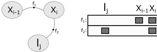
**Fig. 1:** Concept illustration of  $A$ 's structure. Each column represents some variable from state vector. Each row represents some factor from Eq. (1). Factor  $f_1$  of motion model that involves two poses  $x_i$  and  $x_{i-1}$  will have non-zero values only at columns of  $x_i$  and  $x_{i-1}$ . Factor  $f_2$  of observation model that involves together variables  $x_i$  and  $l_j$  will have non-zero values only at columns of  $x_i$  and  $l_j$ .
