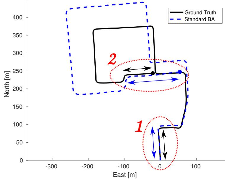
Figure 2.3: Scale drift along optical axis. Top view. Forward-facing camera moves along the trajectory. Black is GT, blue - estimated path. For the 1st 100 frames estimated path is 8% longer than ground truth (zone 1). For the last 100 of frames estimated path is 94% longer than ground truth (zone 2).
