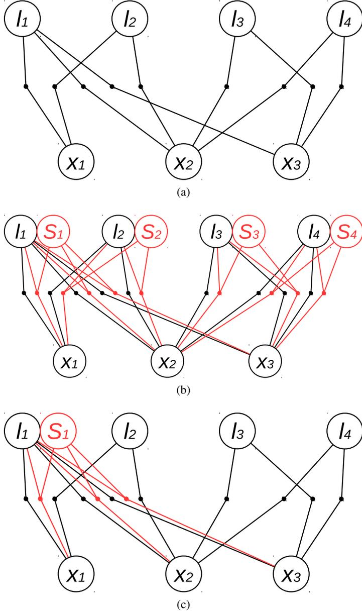
Figure 3.5: Factor graph representations: (a) standard BA with projection factors only; (b) BAFS with naively added all feature scale factors; (c) BAFS with feature scale factors added only for long-term landmarks ( $l_1$ , in this case).
