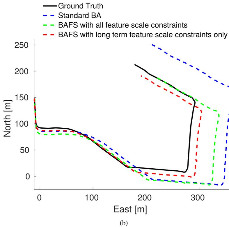
Figure 4.2: Each image provides top view of estimated trajectory for a different KITTI dataset sequence using SIFT features with enhanced scale resolution. Estimation with standard BA is shown with blue, BA + all Feature Scale constraints - green, BA + long term feature scale constraints - red, black solid line is ground truth
