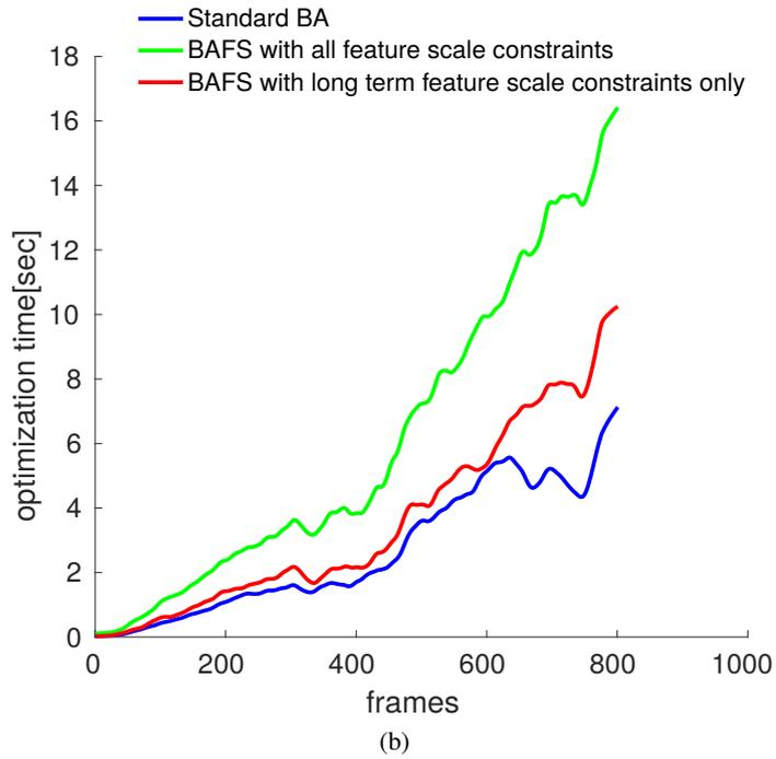
Figure 4.4: Each image provides optimization time for each frame for the 2 different KITTI dataset sequences using SIFT features with enhanced scale resolution. Estimation with standard BA is shown with blue, BA + all Feature Scale constraints - green, BA + long term feature scale constraints - red.
