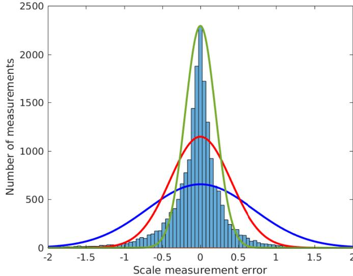
Figure 3.4: Scale error distribution for real images dataset. Red curve is Gaussian curve chosen to approximate data distribution. Green curve over estimates measurements accuracy, blue curve - underestimates.
