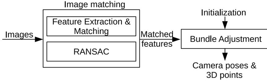
Figure 2.1: Overall framework of monocular BA
