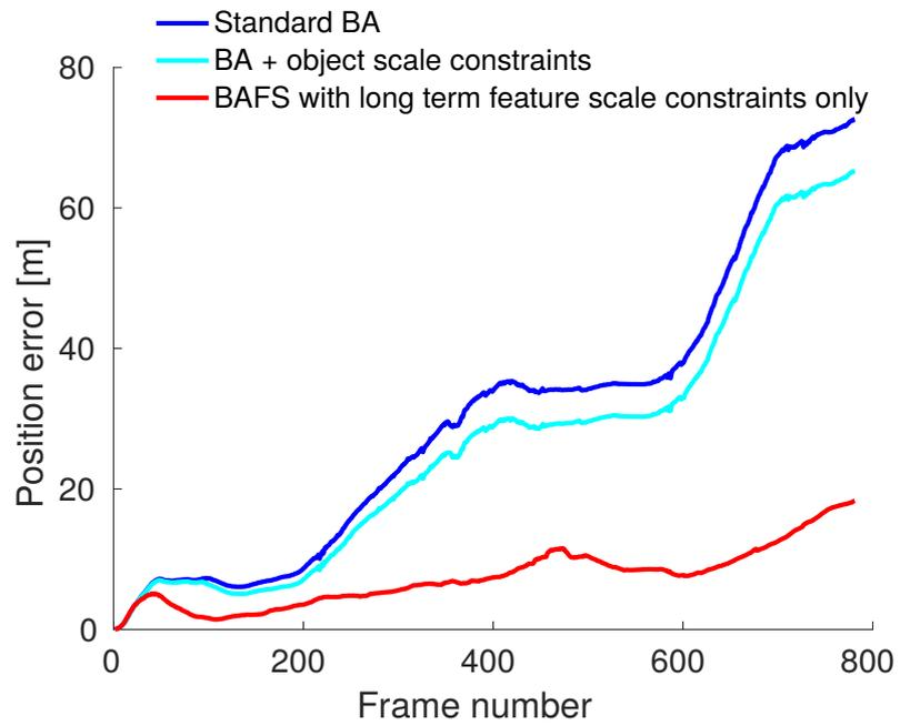
Figure 4.7: Norm of position estimation error as a function of time. Blue - standard BA, cyan - BA with object scale constraints, red - BAFS in modification with long term scale constraints only.
