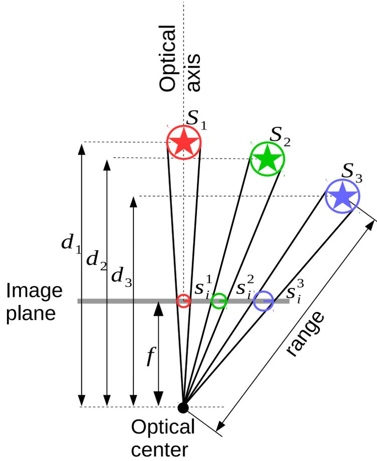
Figure 3.3: Landmark of the same virtual size  $S_j$  is observed at a constant range from the camera's optical center, producing different scale projections depending on the distance along optical axis.
