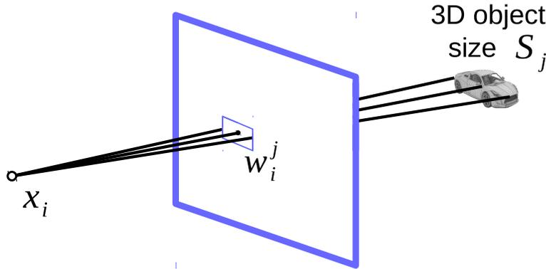
Figure 3.11: Object detected bounding box in the image plane.
