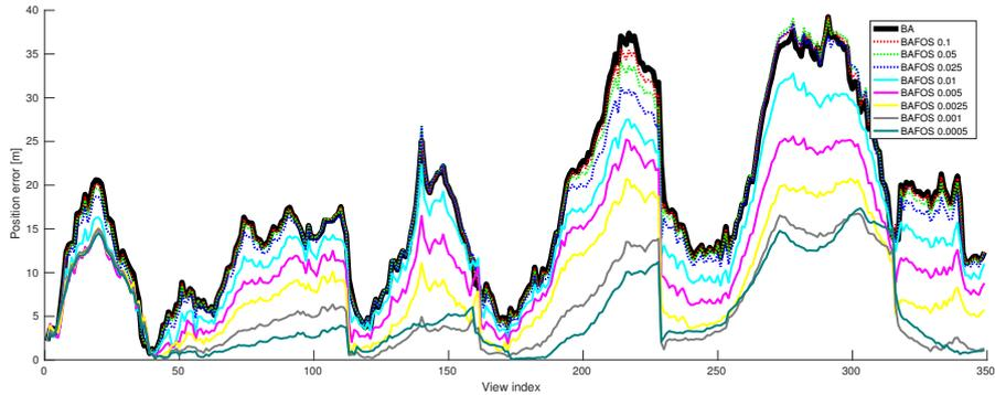
Figure 3.7: Position estimation error. Each curve corresponds to BA with feature scale constraints with noise in simulated feature scale measurements sampled from a Gaussian with different  $\Sigma_{f_s}$ . Black solid curve corresponds to standard BA.
