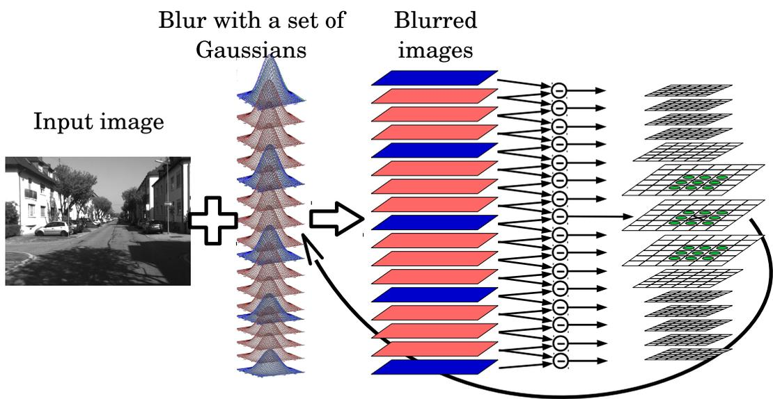
Figure 3.8: SIFT scale estimation process. (i) Blur each input image with a set of Gaussian kernels. (ii) Calculate Difference of Gaussians (DoG). (iii) Feature scale is set as the average of the two Gaussian kernels that correspond to the local-maxima DoG layer.
