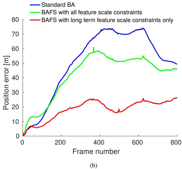
Figure 4.3: Each image provides norm of position estimation error as a function of time for the 2 different KITTI dataset sequences using SIFT features with enhanced scale resolution. Estimation with standard BA is shown with blue, BA + all Feature Scale constraints - green, BA + long term feature scale constraints - red.
