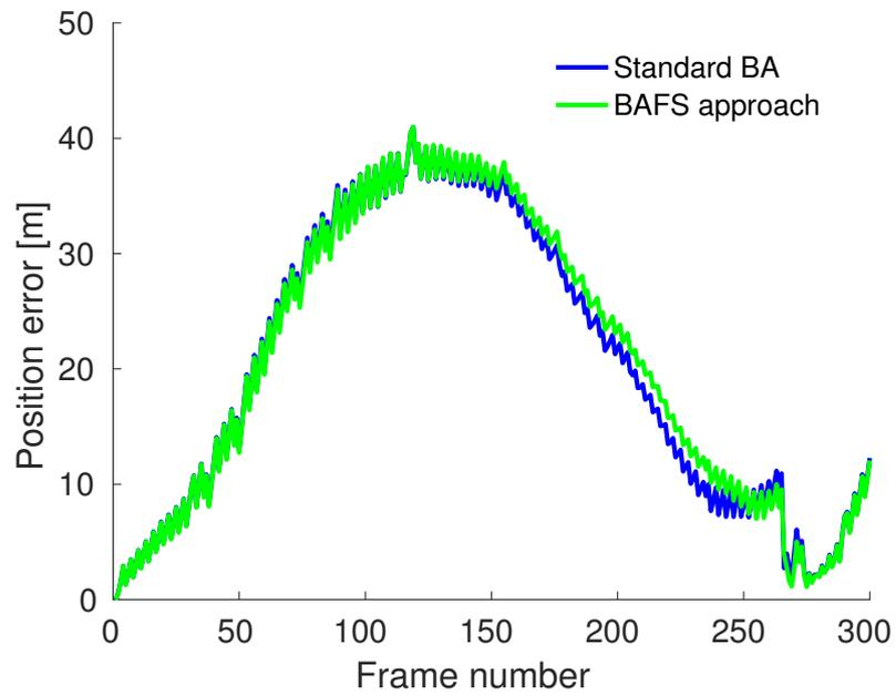
Figure 4.10: Position error for Kagaru dataset as function of time. Estimation with standard BA is shown with blue, BA + Feature Scale constraints - green.
