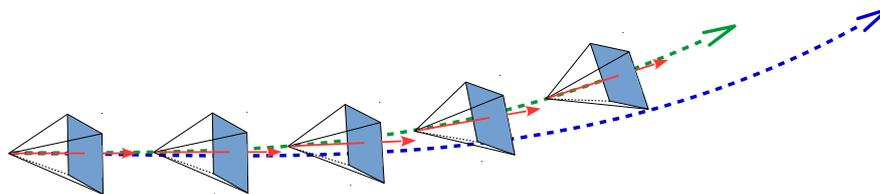
Figure 2.4: Zoomed-in sequence of poses for a single forward-facing camera. Red arrows show camera optical axis direction. Green dashed line is estimated track. Blue line is a ground truth track. Drift along optical axis is cumulative position error component along movement direction.
