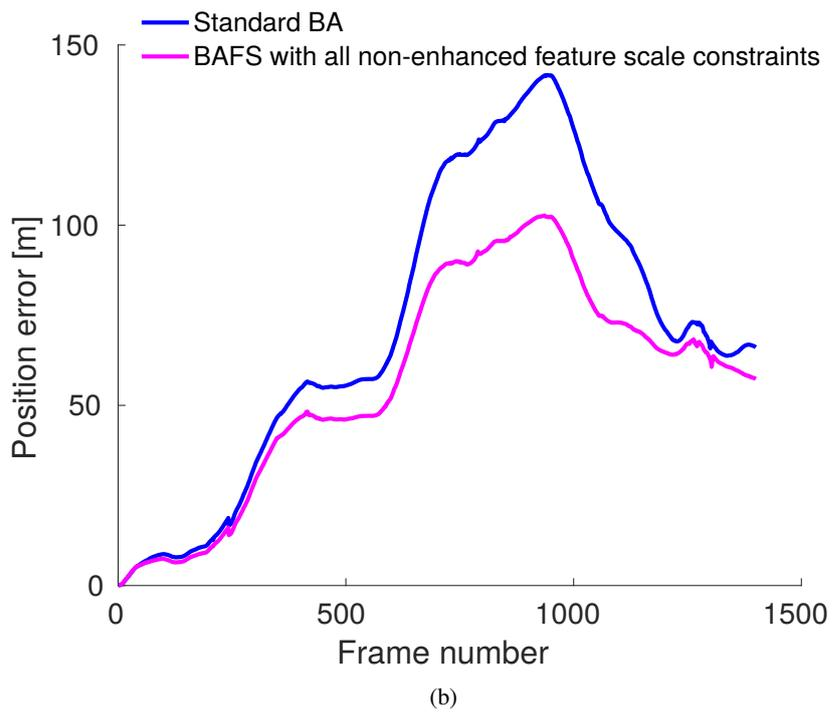
Figure 4.5: (a) image provides top view of estimated trajectory for KITTI dataset sequence using SIFT features with **non-enhanced** scale resolution. Estimation with standard BA is shown with blue, BA + all Feature Scale constraints - magenta, black solid line is ground truth. (b) image provides norm of position estimation error as a function of time using SIFT features with **non-enhanced** scale resolution.
