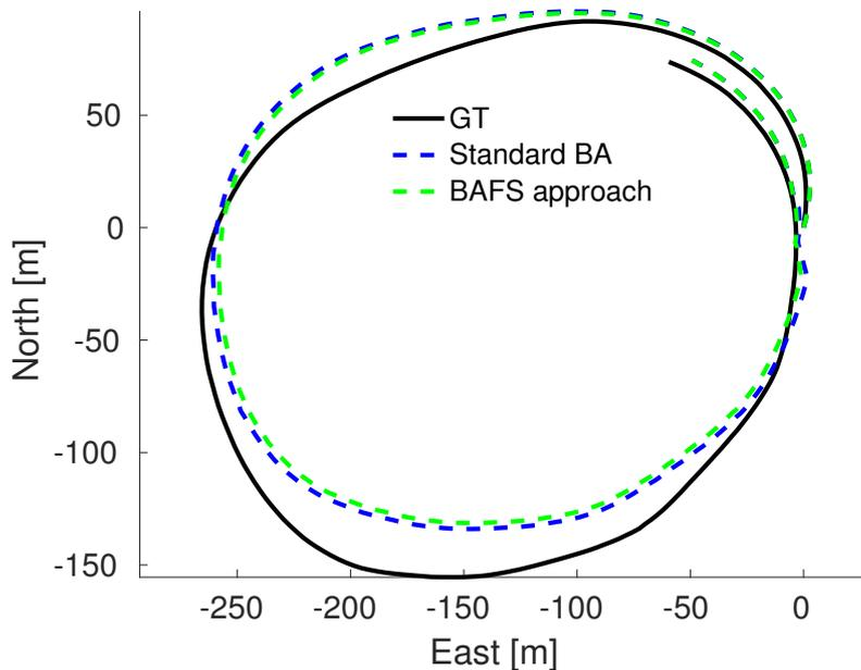
Figure 4.9: Top view of estimated trajectory for Kagaru dataset sequence. Estimation with standard BA is shown with blue, BA + Feature Scale constraints - green, black solid line is ground truth.
