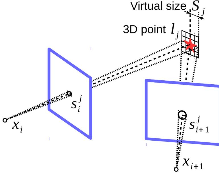
Figure 3.1: Feature scale is modeled as a projection of a virtual landmark size in 3D environment onto the image plane. We leverage the scale invariance property of typical feature detectors, according to which, detected scales of matched features from different images correspond to the same virtual landmark size in the 3D environment, and incorporate novel feature scale constraints within BA.
