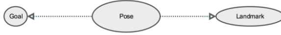
Figure 1. Schematic of an infeasible planning problem. The landmark uncertainty is high enough to deny the robot sufficient localization after loop-closure, while moving directly towards the goal fails to contain the uncertainty within a maximum allowed limit.
