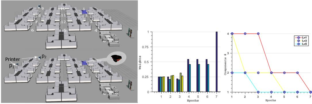
Fig. 5: (top) The aliased 2 floor office room environment in a Gazebo simulator with Pioneer. Here,  $p_1$  and  $p_2$  denote the printers; 1, 6 are the mean positions in each floor for the 4-modal initial GMM belief. (bottom left) Evolution of weights of the components in the GMM after inference for  $L = 2$ . (bottom right) Average number of components in the belief mixtures for different planning horizon.
